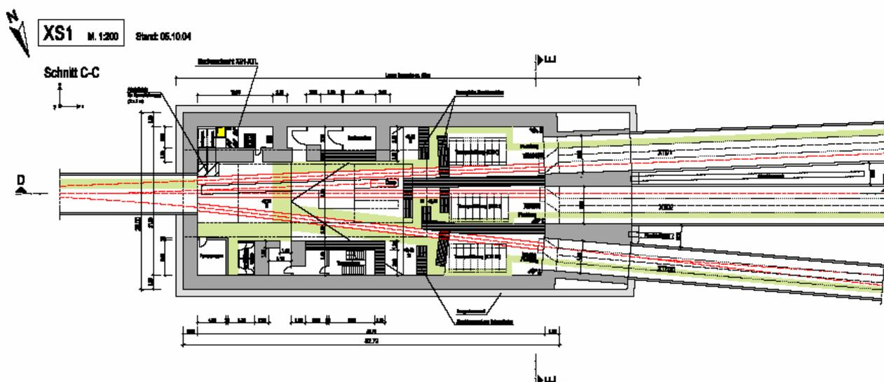
**Figure A3.6:** Top view of the XS1 beam distribution shaft. The linac tunnel is to the left. The upper two tunnels to the right belong to the SASE-1 and SASE-2 beamlines of the phase-I development, the lower tunnel branches off to the later phase-II of the facility.
