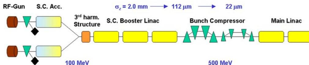
**Figure A3.3:** Injector Layout
