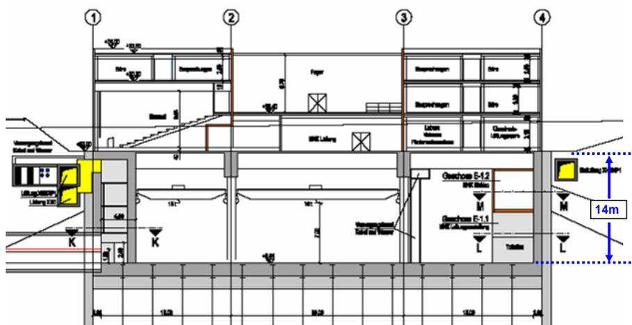
**Figure A3.7:** Side view of the experimental hall (photon beam lines are to the left) and of the surface building on top.
