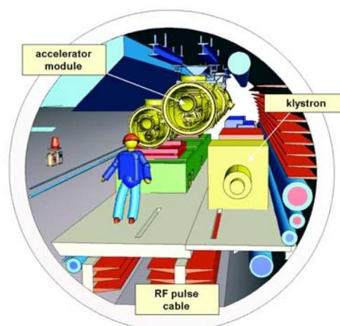
**Figure A3.5:** Sketch of the 5.2m diameter main linac tunnel. The accelerator modules will be suspended from the ceiling.
