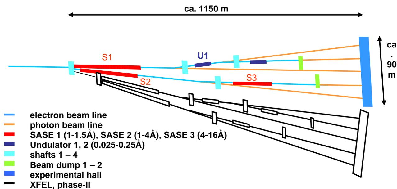
**Figure A3.1:** The phase-I user beamline layout (coloured) and the possible phase-II extension.
