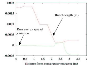
The bunch compression does not significantly impact the beam quality (projected transverse horizontal emittance growth is kept at about 10 % and slice emittance is not significantly affected)
