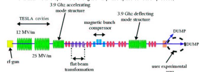
The proposed upgrade for A0-photoinjector : "a ~1/4 scaled version of the X-FEL" injector
