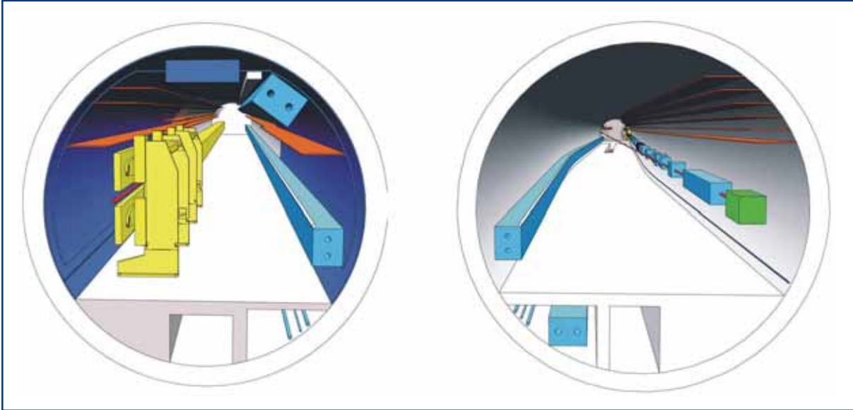
Figure 7.1.16 Cross sectional view of the tunnel in the region of the SASE undulators as viewed in the beam direction. The diameter of the tunnel is determined by the transport path for a replacement undulator module and the necessary emergency pathway (see position A-A in Figure 7.1.15).
