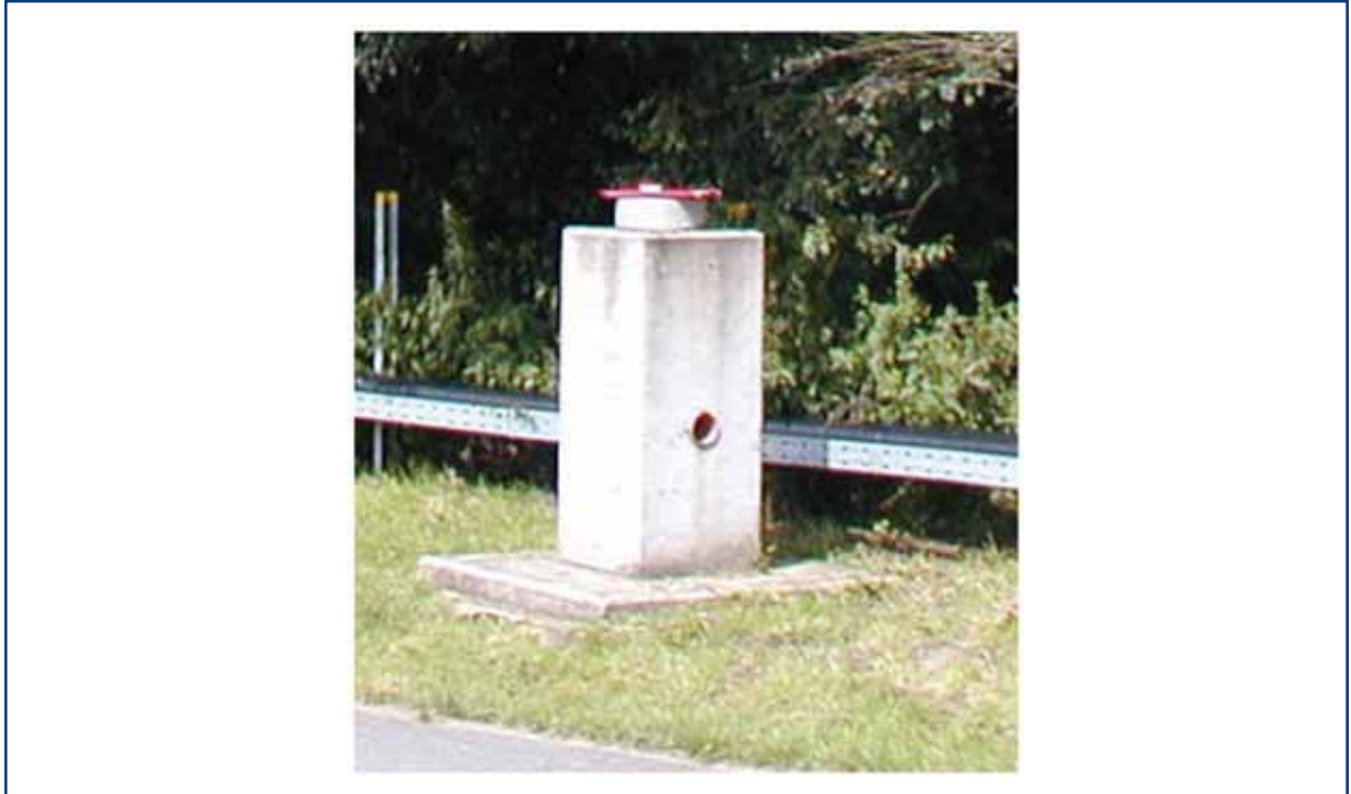
Figure 7.2.8 Survey reference monument.
