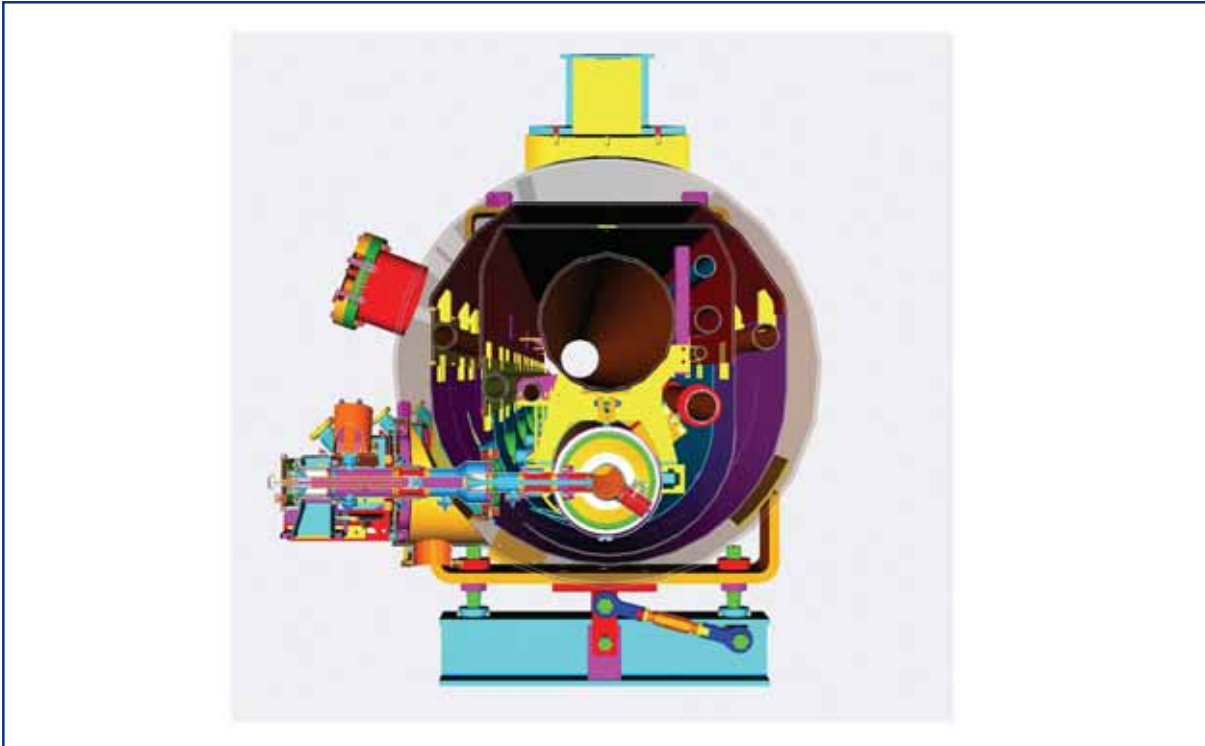
Figure 4.2.15 Cross-section of a type-3 cryomodule.
